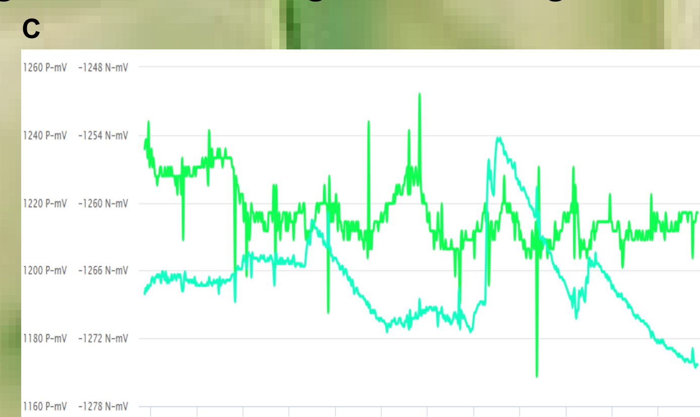
Figure 1. Continuous monitoring of (A) dendrometry data (trunk expansions and dilations), (B) moisture values in the soil profile and (C) Potassium and nitrate potential. Source : Globalsens Platform
